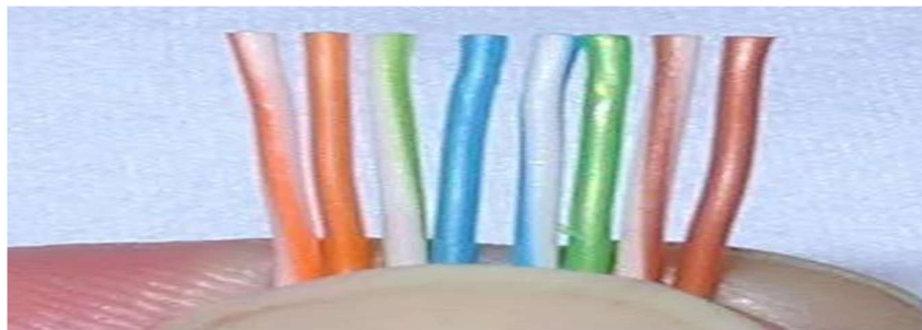
Figure 1.6: Cable cut into same length
